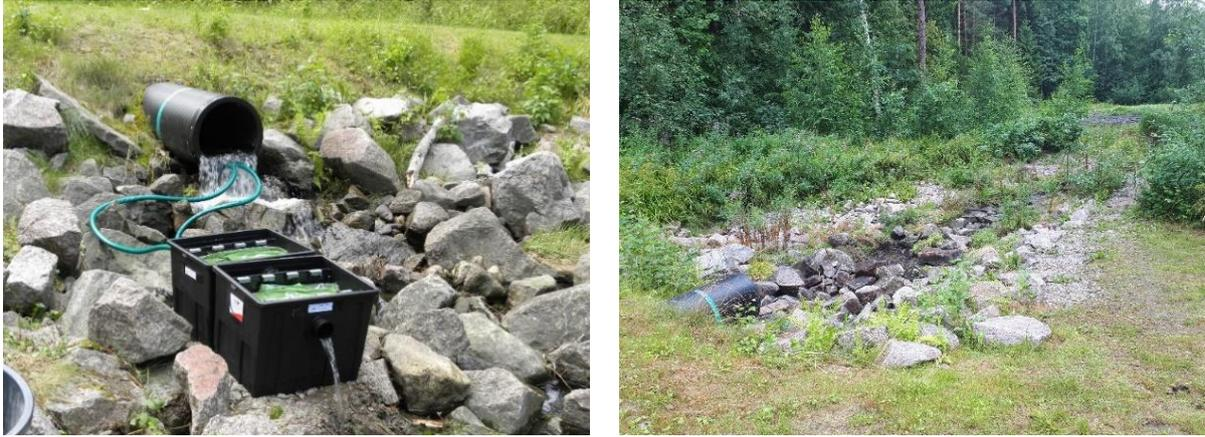
Figure 42 Pre-test filter located at outlet of 1<sup>st</sup> basin at Sammonlahti constructed wetland
