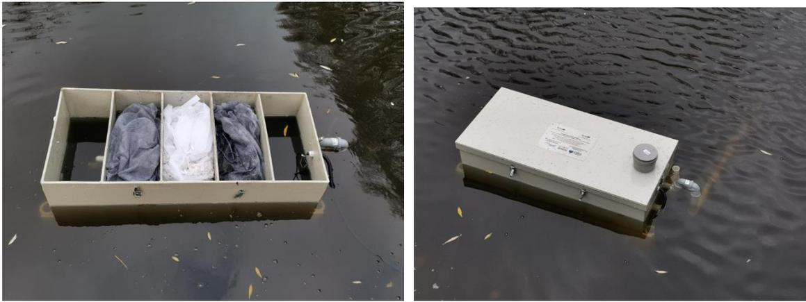
Figure 30. Installation of sorption filter equipped by water pump.
