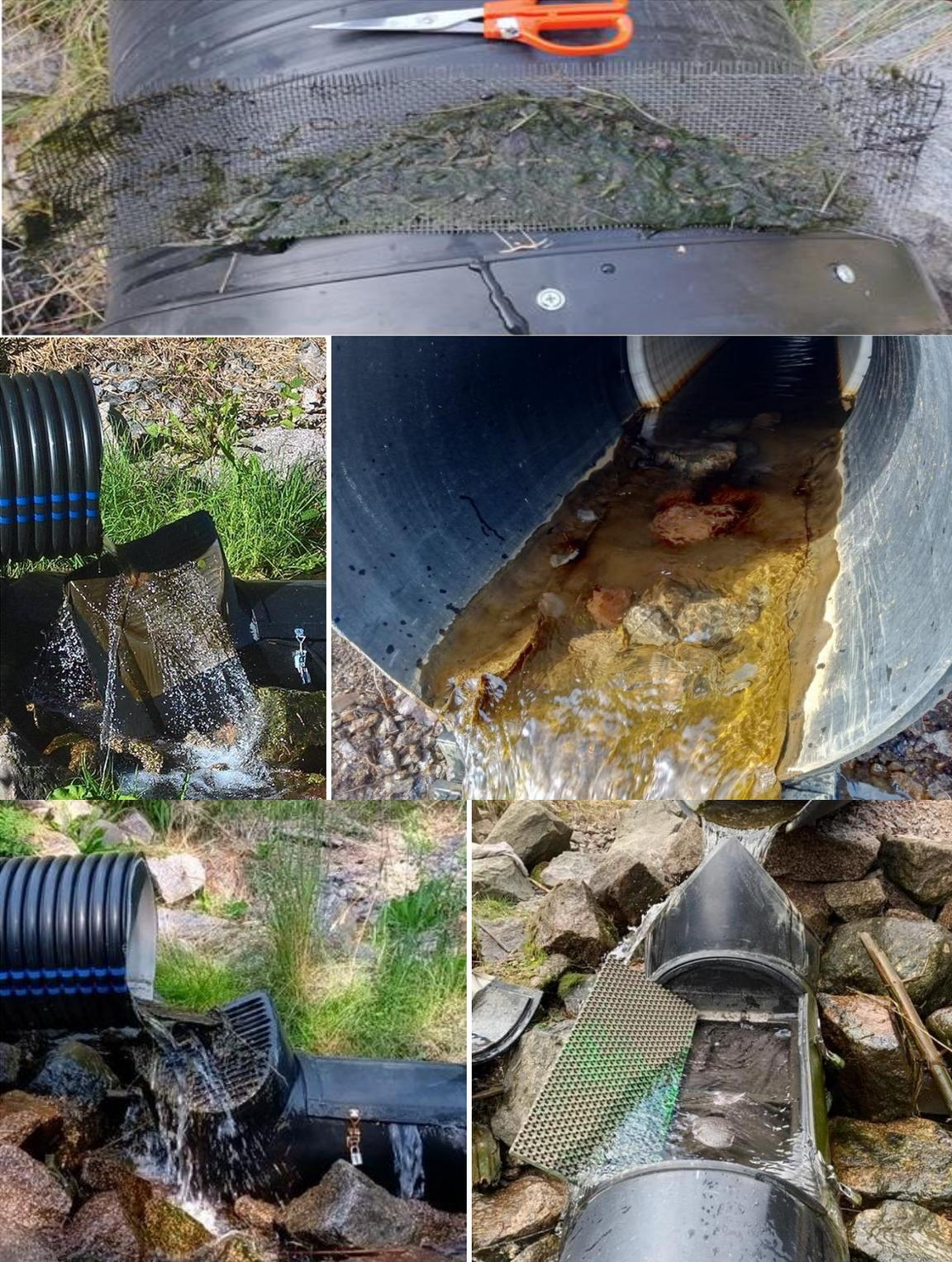
Figure 59 Visualization of common clogging and flow issues in field tests: a) organic matter clogging the pre-filter mesh, B) too tight mesh as pre-filter blocks the flow, c) melting water brought stones into filter, D) floating material is a problem, F) filter opened after winter is functioning without problems.
