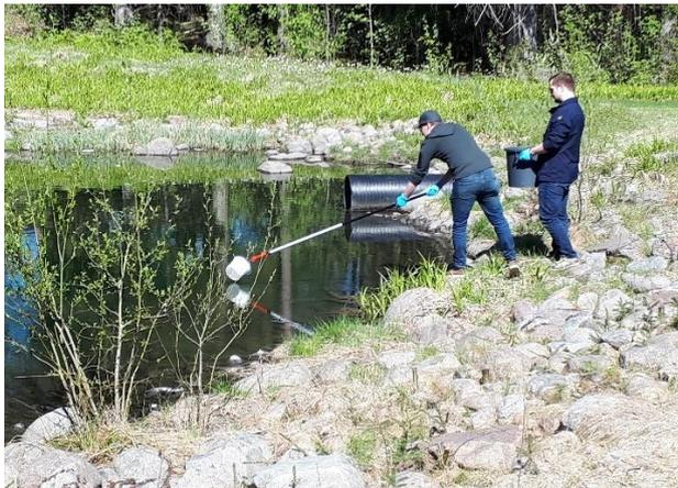
A) Sammonlahti Basin 1 and 2 water samples were taken as composite samples of 5-10 subsamples. The depth of water was typically 50 +/- 20 cm.
