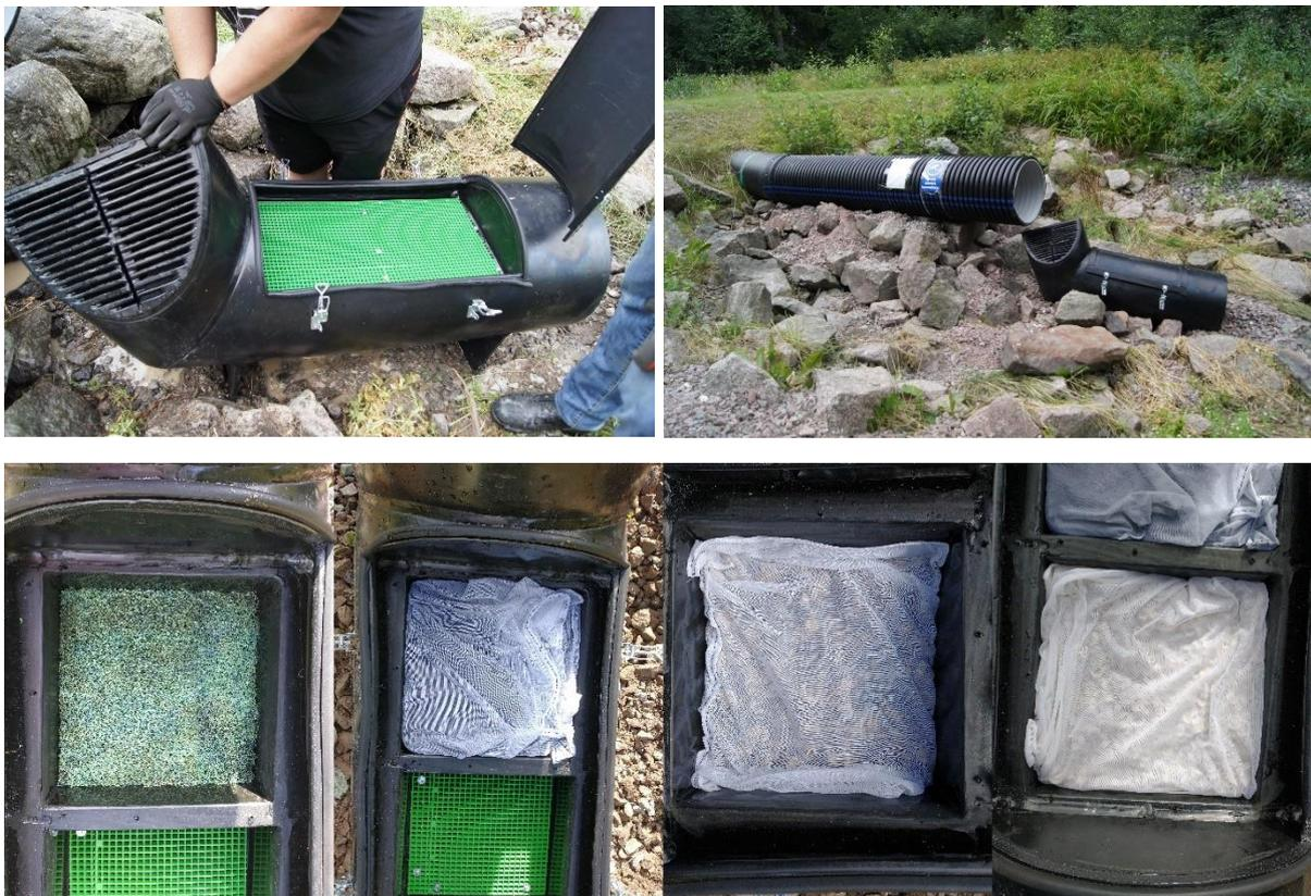
Figure 35 Vertical flow filter applied in Sammonlahti CW at 2020-2021 field test.
