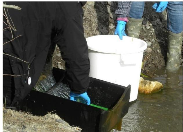
D) Shungite samples from filters were collected for adsorption studies.
