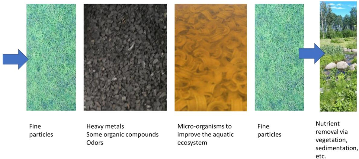
Figure 31 Filters consist of foam to filter fine particles, and two chambers: one for shungite and other one for EM growth media. The settlement pool(s) after the filter system are counted as essential part of the proposed purification system.
